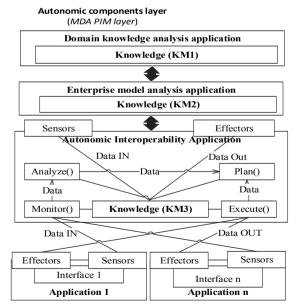
Fig. No. 12. The architecture of the interoperable enterprise applications.
