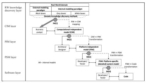
Figure No. 4. The modified MDA schema includes two modeling paradigms.
