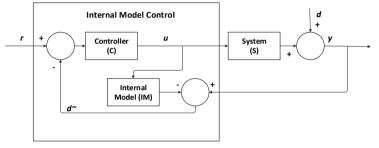
Figure No. 1. The internal model-based control system.
