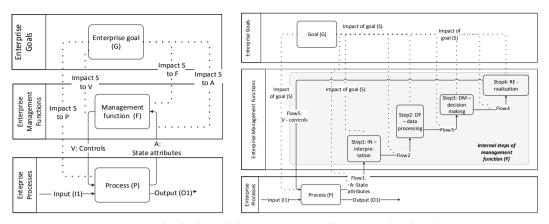
*Figure No.* **6.** *The knowledge components of an enterprise domain: b) Adopted for enterprise software engineering MT and EMC frameworks (BPMN notation).*
