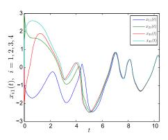
**Figure 3.** The state trajectories  $x_{i1}(t)$  of four agents under the control protocol (2).
