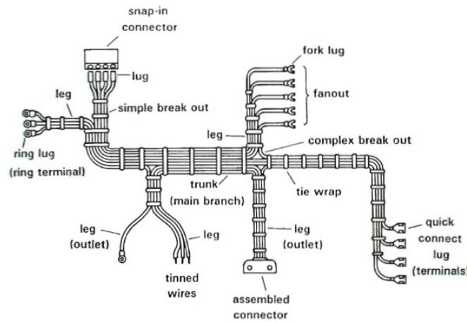
Fig. 1. The main wiring harness components and terminology [13].
