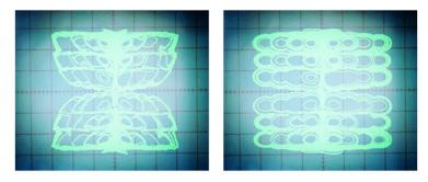
Fig. 13. Circuit experimental results of grid multi-wing chaotic attractors on the xz-plane, yz-plane: 8×6-wing.
