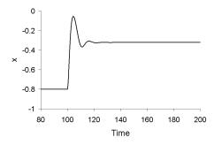
Fig. 2. One-step stabilization of the UFP of the Duffing oscillator given by Eq. (14). The control is switched on at t=100. The parameters are  $b=0.5,\,k=1.1$ . SFP observed before switching the control  $x_{01}=-0.8$ , extracted unknown term  $\xi=x_{01}^3-x_{01}=0.288$ , stabilized UFP and coordinate calculated from the formula (25)  $x_{02}=-0.321$ .
