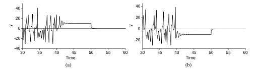
Fig. 5. Two-step stabilization of the saddle UFP in the Lorenz system given by Eqs. (22), (23). The first step is switched on at t=40, the second step is applied at t=50. The parameters are  $\sigma=10$ ,  $\beta=8/3$ ,  $k_1=10$ ,  $r_1=0$ . The z-coordinate of the artificial SFP  $z_{12}=z_{13}=39$ , the extracted unknown parameter  $\xi=z_{12}+k_1+1=50$ ,  $k_2=60$ . The stabilized UFP (0,0,0). Initial conditions: (a) x(0)=0.10, y(0)=z(0)=0; (b) x(0)=0.11, y(0)=z(0)=0.
