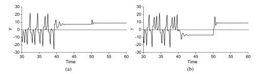
Fig. 4. Two-step stabilization of the spiral UFP in the Lorenz system given by Eqs. (22), (23). The first step is switched on at t=40, the second step is applied at t=50. The parameters are  $\sigma=10$ ,  $\beta=8/3$ ,  $k_1=k_2=10$ ,  $r_1=0$ . The z-coordinate of the artificial SFP  $z_{12}=z_{13}=19$ , the extracted unknown parameter  $\xi=z_{12}+k_1+1=30$ , the stabilized UFP (8.79, 8.79, 29.0). Initial conditions: (a) x(0)=0.10, y(0)=z(0)=0; (b) x(0)=0.11, y(0)=z(0)=0.
