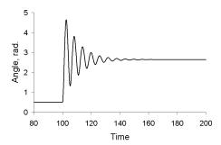
Fig. 1. One-step stabilization of the upper position of mechanical pendulum given by Eq. (10). The control is switched on at t=100. The parameters are  $\beta=0.2, k=2$ . The stable angle observed before switching the control  $\varphi_{01}=0.5$ , extracted unknown term  $\xi=\sin\varphi_{01}=0.47943$ , stabilized UFP and angle calculated from the relationship  $\varphi_{02}=\pi-\varphi_{01}=2.64$ .
