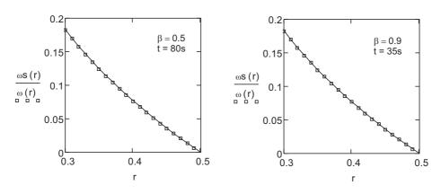
Fig. 1. The time after which the diagrams of w(r,t) are almost identical to those of  $w_s(r)$ , for f = -2,  $R_1 = 0.3$ ,  $R_2 = 0.5$ ,  $\nu = 0.001188$ ,  $\mu = 1.05$ ,  $\alpha = 0.002$ ,  $\beta = 0.5$  and 0.9.
