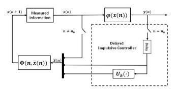
Figure 1. Schematic of delayed impulsive control systems.
