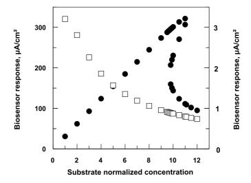
Fig. 3. The dependence of biosensor response on normalized bulk concentration of substrate. The data calculated with  $\rho=30$  ( $\bullet$ ) belongs to left hand y axis, with  $\rho=0.3$  ( $\square$ ) – to right hand y axis.
