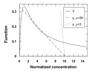
Fig. 1. Graphical surface concentration calculation. Functions:  $Y = c_s/(1 + c_s + c_s^2)$ ,  $y = (c_b - c_s)/\rho$ . The parameters of calculations are written in the text.
