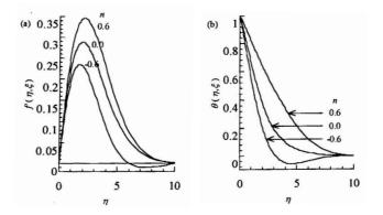
Fig. 5. (a) The velocity distribution and (b) the temperature distribution for different values of n with the selected Prandtl number Pr = 0.708 and  $\xi = 0.6$ .
