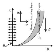
Fig. 1. The flow configuration and co-ordinate system.
