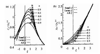
Fig. 2. (a) Dimensionless skin-friction and (b) dimensionless heat-transfer for different values of  $\xi$  as well as n with the selected Prandtl number Pr = 0.708.
