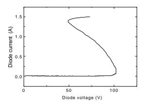
Fig. 3. Calculated current - voltage characteristic of the diode.
