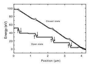
Fig. 4. Potential (the edge of  $\Gamma$  valley and the top of heavy hole subband) distributions in the low and high conductance states. The results were obtained under the same conditions as in Fig. 3 and correspond to the time moments t = 90 ps for the low conductance state, and to t = 130 ps for the high conductance state, respectively. The upper and lower arrows indicate the regions in which an intensive impact ionisation is initiated by electrons and holes, respectively, in the open state.
