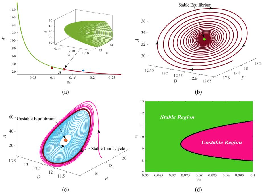
**Figure 8.** (a) Bifurcation diagram in the  $q_{11}A^*$ -plane with the corresponding stable limit cycle in the  $q_{11}DA$  space with  $H$  denoting the Hopf point; (b), (c) phase portraits in the  $DPA$ -space for  $q_{11} = 0.1$  and  $0.18$ , respectively (green dot: stable equilibrium, red dot: unstable equilibrium); (d) stable and unstable regions of the coexisting equilibrium  $E^*$  in the  $q_{11}m$ -plane. Remaining parameters are same as in Table 1.
