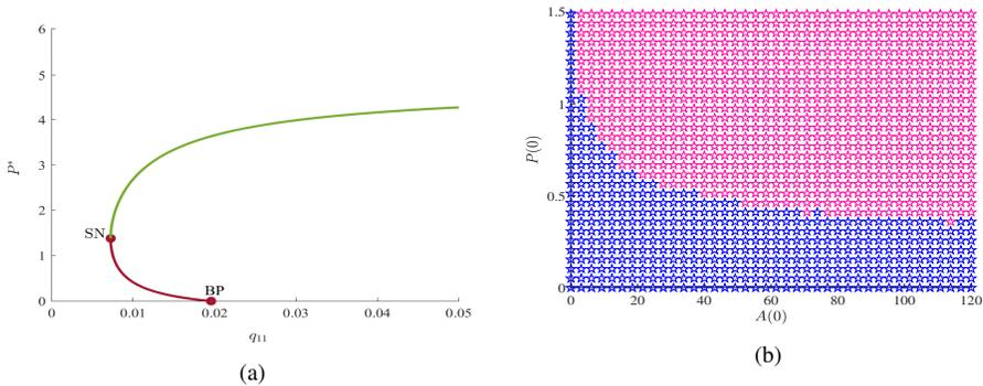
**Figure 9.** (a) Equilibrium curve showing a saddle-node bifurcation with respect to  $q_{11}$  for  $\alpha_1 = 0.023$  with *SN* and *BP* marking the saddle-node and transcritical bifurcation points, respectively; (b) basin of attraction in  $A(0)P(0)$ -plane. Remaining parameter values are same as in Table 1.
